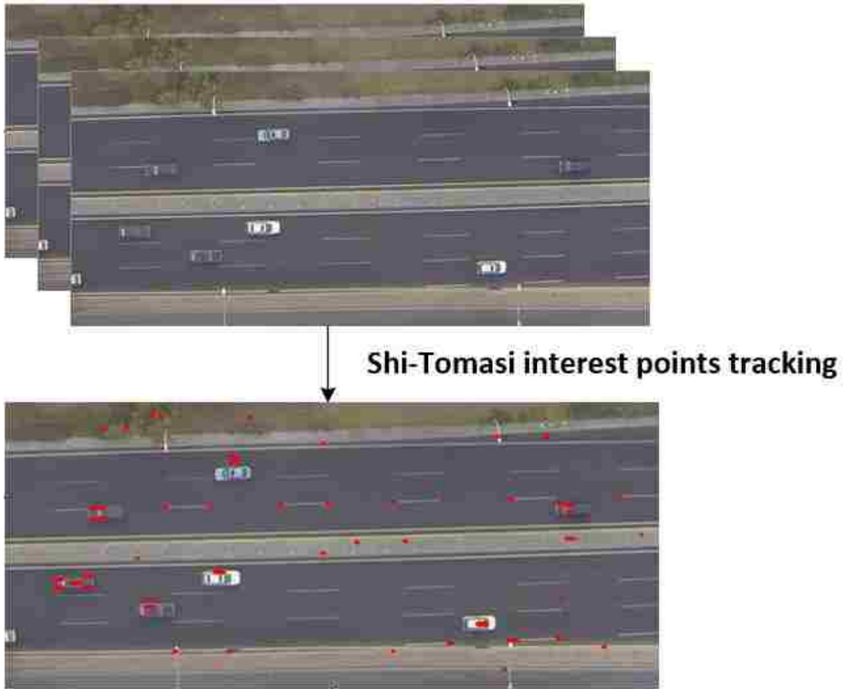
Figure 3-2 Optical flow-based Shi-Tomasi interest points extraction and tracking
