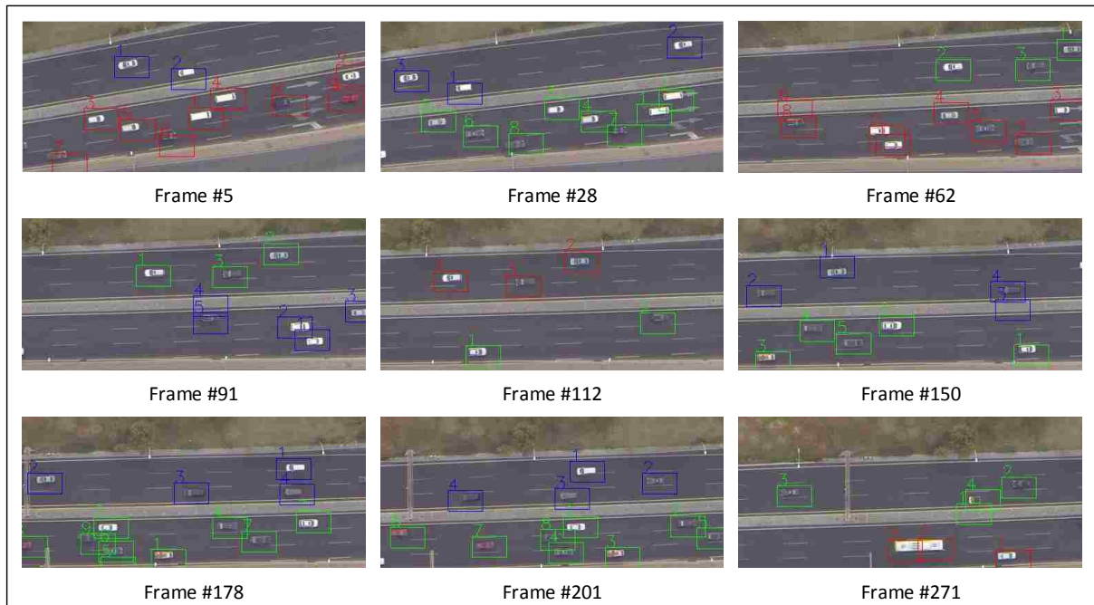
Figure 6-2 Selected frames showing the bi-directional vehicle counting results
